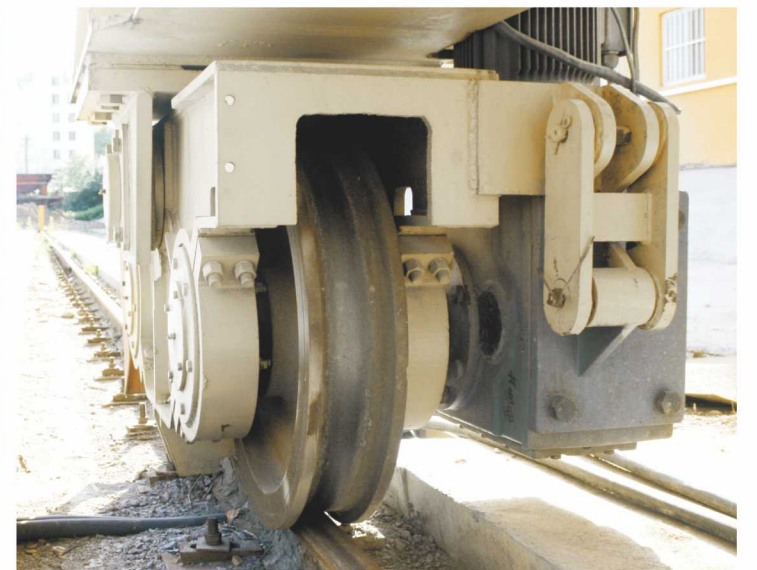
42CrMo alloy forged wheel wear resistance, impact resistance, high performance, long life span.
