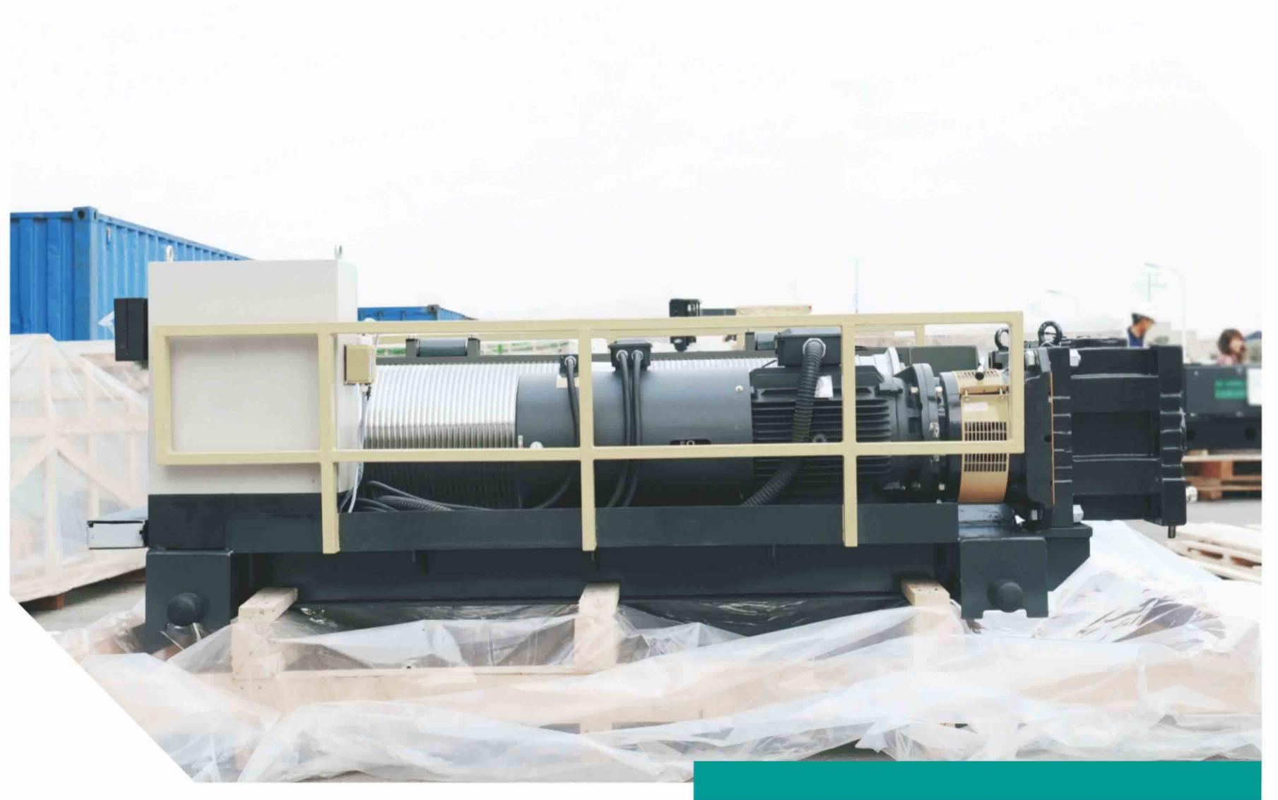
Hard teeth gearbox is designed to adapt to frequent and heavy working conditions. The low speed axle is connected with the drum directly and gears of all levels are hardening treated helical gears. Long-acting lubrication is realized by oil bath to ensure higher abrasion resistance and quiet running.
