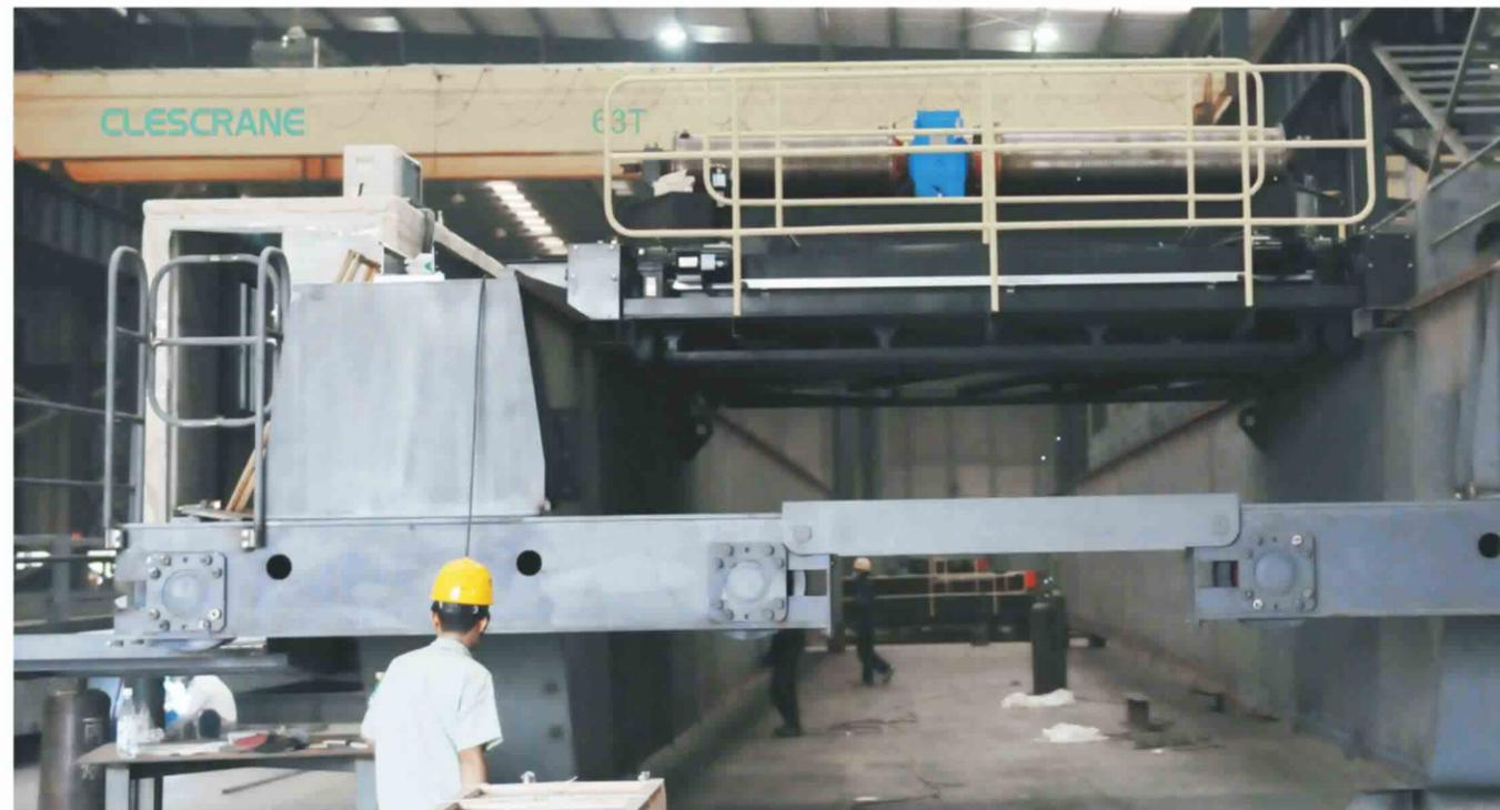
Holistic processing technology is adopted on end carriages whose processing accuracy ensures the assembly accuracy between wheel groups and end carriages. Easy maintenance allows the operator do daily check quickly according to random product manual. Because of the adoption of modular parts, the requirement on regular maintenance is low. Common maintenance staff can do it quickly.
